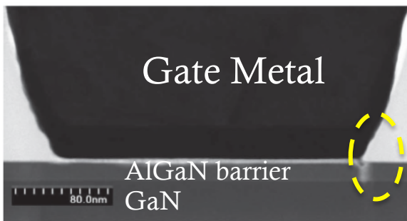
Figure 4-47 (left) Z-contrast images of a stressed devices. Material below the horizontal interface is semiconductor; the trapezoidal shape defines the gate metal. Right side is toward the drain, and left side is toward the source in all three images. Figure shows a severe case of degradation where the gate metal (Pt) has diffused into the crack formed (from [Chowdhury2008]). (right) Schematic drawing of the gate edge degradation mechanisms
